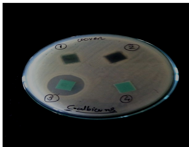
Figure-2 Zone of inhibition ( Candida albicans ) of 100% Cotton woven coated fabric
