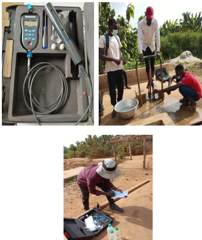
Figure-4: AQUAREAD AP-700 multi-parameter and in-situ parameter measurements.
