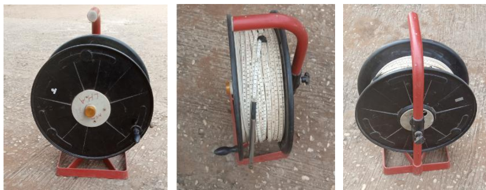
Figure-3: Various views of a piezometer probe for static measurement of the water table.
