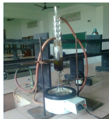
Figure-1 Photograph showing extraction of leaves of Mimusops elengi using soxhlet apparatus
