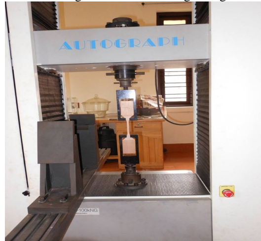
Figure-1 to 8 Testing of Mechanical Properties of Melia dubia by Universal Timber Testing Machine
