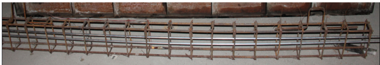
Figure-1 Duct with non-prestressed steel reinforcement
