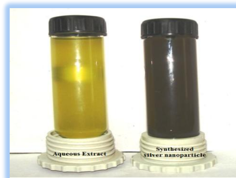
Figure 2 Aqueous extract of Hibiscus rosasinensis leaves and the synthesized silver nanoparticle solution
