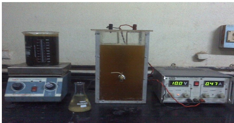
Figure-1 Experimental Setup for colour removal using adsorption and EC
