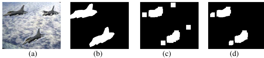
Figure-4 Examples of CRM forgery and its detection result: (a) the forged image by CRM forgery of 10, (b) forged region, (c) detected region, and (d) (forged region \cap detected region) 4
