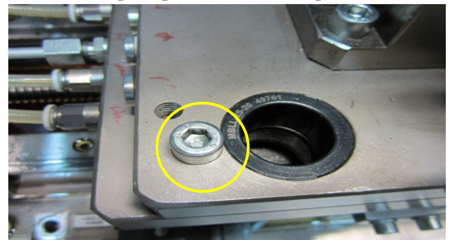
Figure-3 Remove the four holding screws (step iii) and two alignment screws (step ix)
