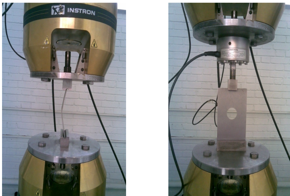
Figure-7 The setup of experimental tests (in this case, both of the supports are simply)
