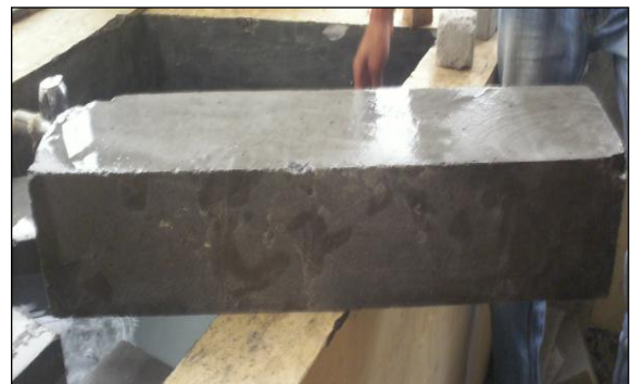
Figure-4 Beam specimen
