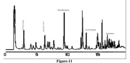
BTEX fingerprints of the oil extract before treatment with the oxidants
