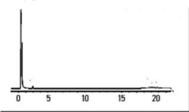
Figure-12 Chromatogram showing the BTEX concentration of the soil sample after treatment with potassium persulfate at the acidic pH range
