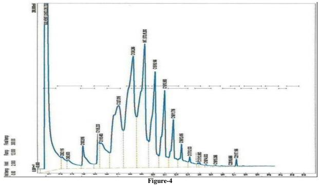
TPH components after treatment with persulfate at the basic pH medium
