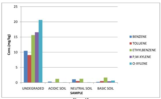
Figure-15 Chart showing depletions of the BTEX components of the samples at the different pH media after treatment with potassium persulfate
