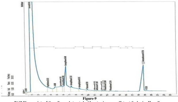
PAH Fingerprints of the soil sample treated with potassium persulfate at the basic pH medium
