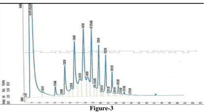
TPH components of the soil treated potassium persulfate at the neutral pH medium
