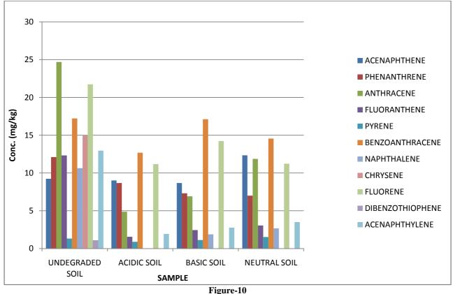
Chart showing the extent of depletion of PAH components of the sample at different pH media after treatment with potassium persulfate
