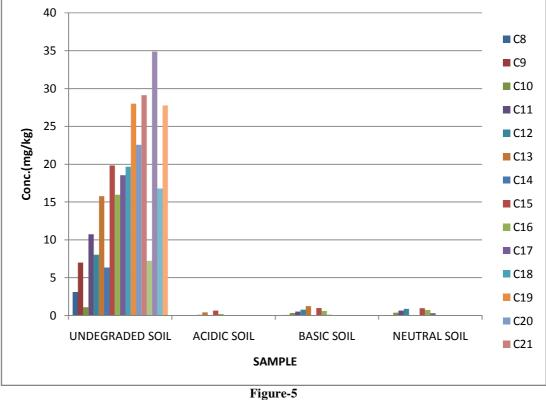
Chart showing extent of TPH depletion of the samples after treatment with potassium persulfate at the various pH ranges
