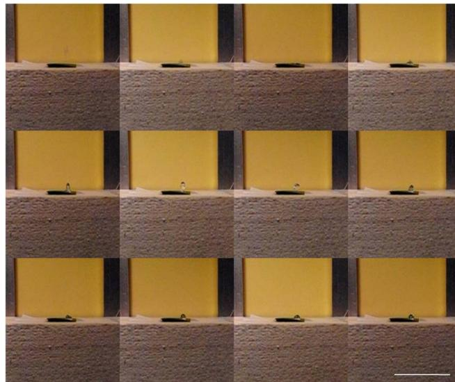
**Figure-15:** Drop impacts on *Lactuca virosa* (Wild lettuce) surface. (Needle to sample length 75mm, scale bar 1cm,  $V=4\text{m/s}$ ).
