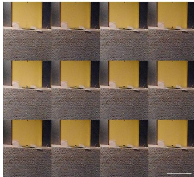
**Figure-12:** Drop impacts on *Leucophyllumfrutescens* (Purple Sage) surface. (Needle to sample length 35mm, scale bar 1cm,  $V=2\text{m/s}$ ).
