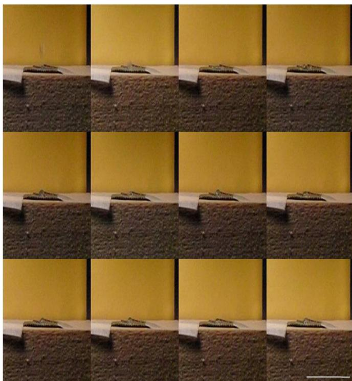
**Figure-11:** Drop impacts on *Corymbia* (Eucalyptus) surface. (Needle to sample length 70mm, scale bar 1cm,  $V=4\text{m/s}$ ).
