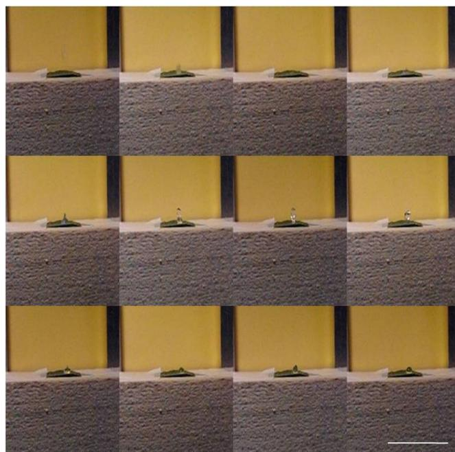
**Figure-13:** Drop impacts on *Leucophyllumfrutescens* (Purple Sage) surface. (Needle to sample length 70mm, scale bar 1cm,  $V=4\text{m/s}$ ).
