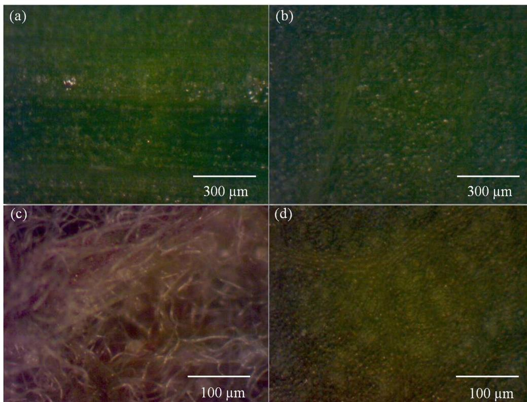
**Figure-5:** Microscopic images of the natural leaves. (a) Small horizontal lines were appeared on *Montbretia* (*Crocasmia*) leaf (b) On *Corymbia* (*Eucalyptus*) surface, small dots were observed (c) shows a brownish surface on (*Leucophyllum frutescens*) (Purple sage), heavily covered with three dimensional hair (d) shows *Lactuca virosa* (Wild lettuce) surface with tiny dots.
