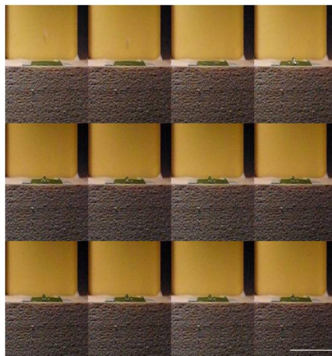
**Figure-9:** Drop impacts on *Montbretia* (*Crocasmia*) surface (Needle to sample length 70mm, scale bar 1cm,  $V=4\text{m/s}$ ).
