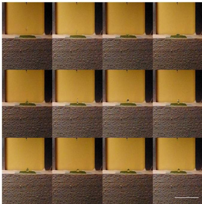
**Figure-8:** Drop impacts on *Montbretia* (*Crocasmia*) surface. (Needle to sample length 35mm, scale bar 1cm,  $V=2\text{m/s}$ ).
