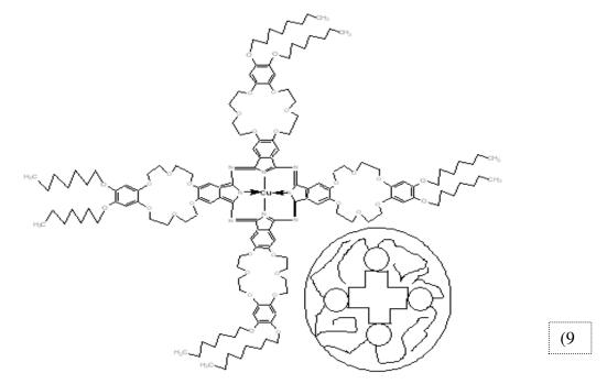
Long alkyl group crown ether substituted phthalocyanines. Also used as in the photovoltic cells
