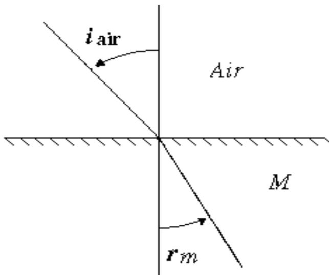
(Refraction of a ray of light on passing from air into medium M) In short, the bending of a ray of light on passing from one medium to another is called refraction.
