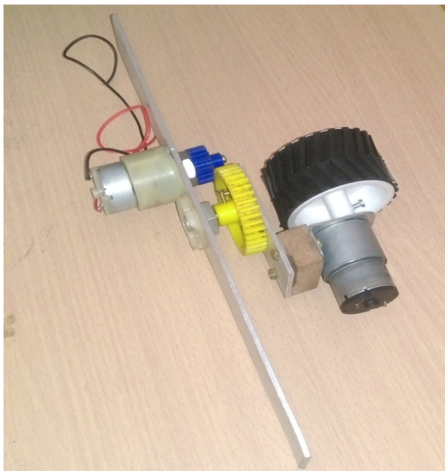
Figure-3: One side assembly fixed on aluminium strip.
