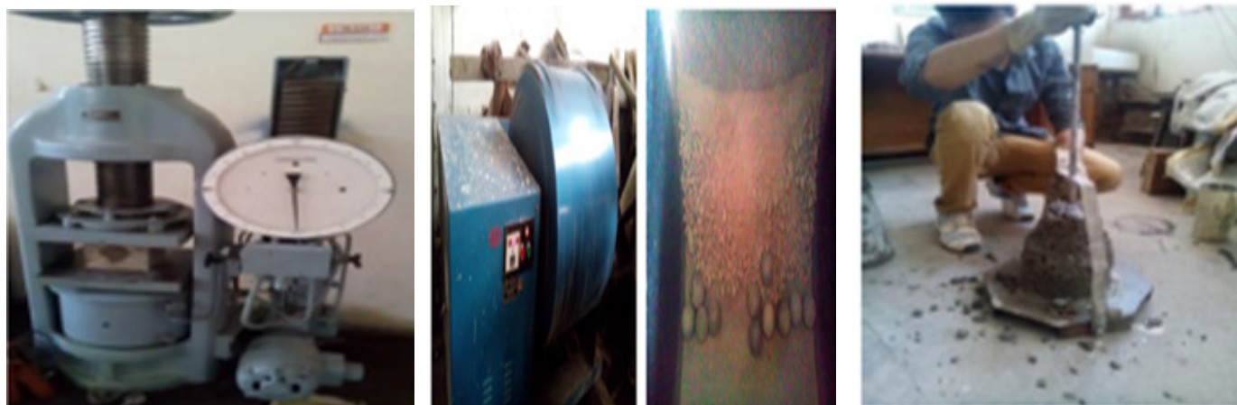
Figure-5: (a) Compressive Strength Test, (b,c) Los Angeles Abrasion Test, (d) Slump Cone Test.
