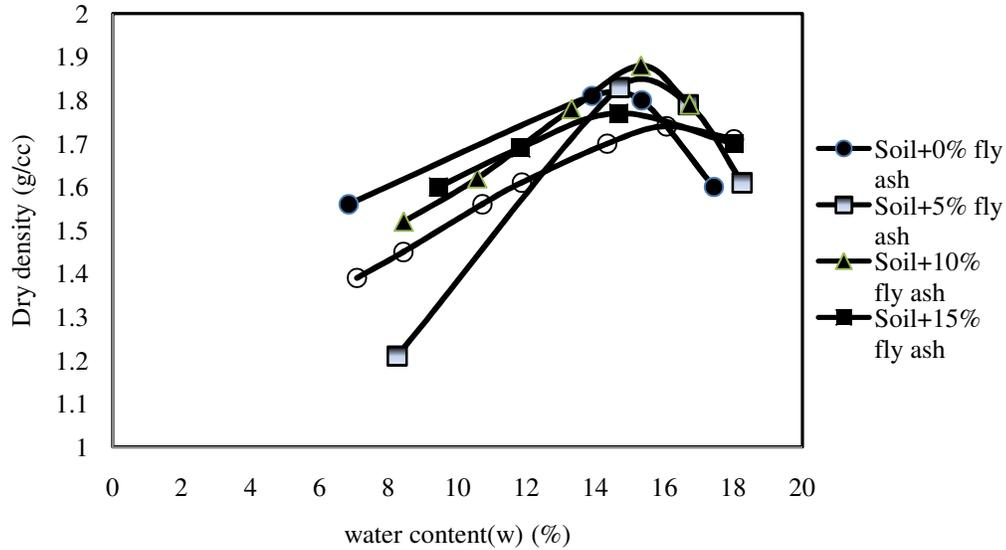
Figure-3(a): Compaction curve for Soil and Fly ash Mixture.
