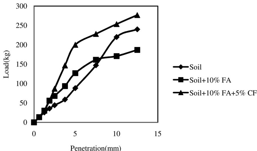
Figure-5(c): Comparison of Load-penetration curve of Soaked CBR.
