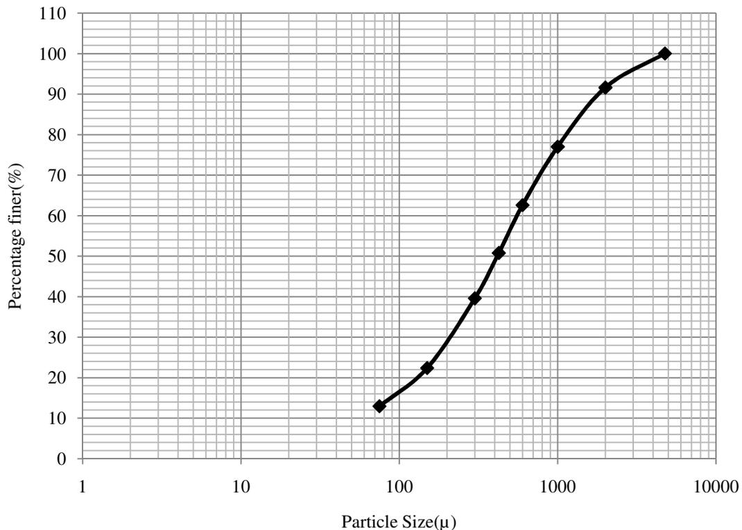
**Figure-1:** Particle Size Distribution Curve of Soil.
