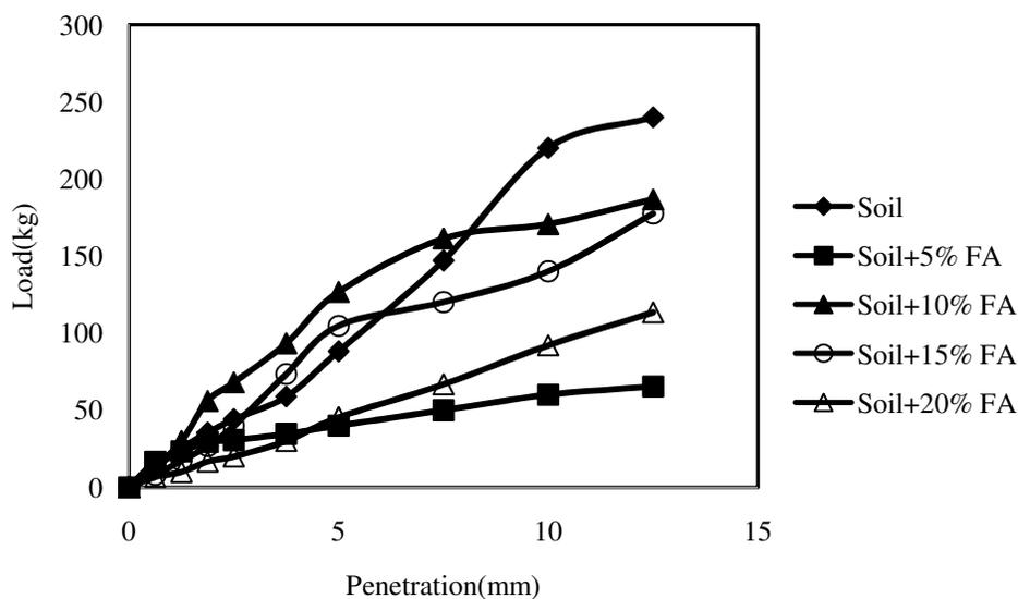
**Figure-5(a):** Load-Penetration Curve for Soil and various Fly Ash contents.
