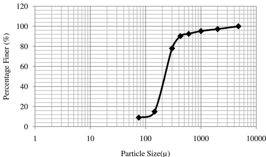
**Figure-2:** Particle Size Distribution Curve of Fly ash.
