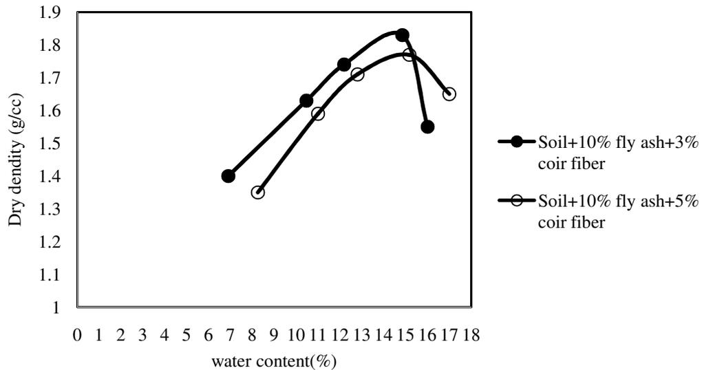
Figure-3(b): Compaction Curve for Soil, Fly ash and Coir fiber mixture.
