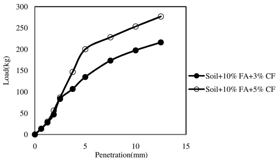
**Figure-5(b):** Load-Penetration Curve for Soil, Fly ash and various percentage of Coir Fiber.
