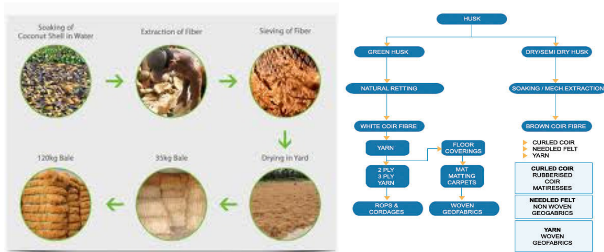
Figure-2 Flow Diagram of Coir Production
