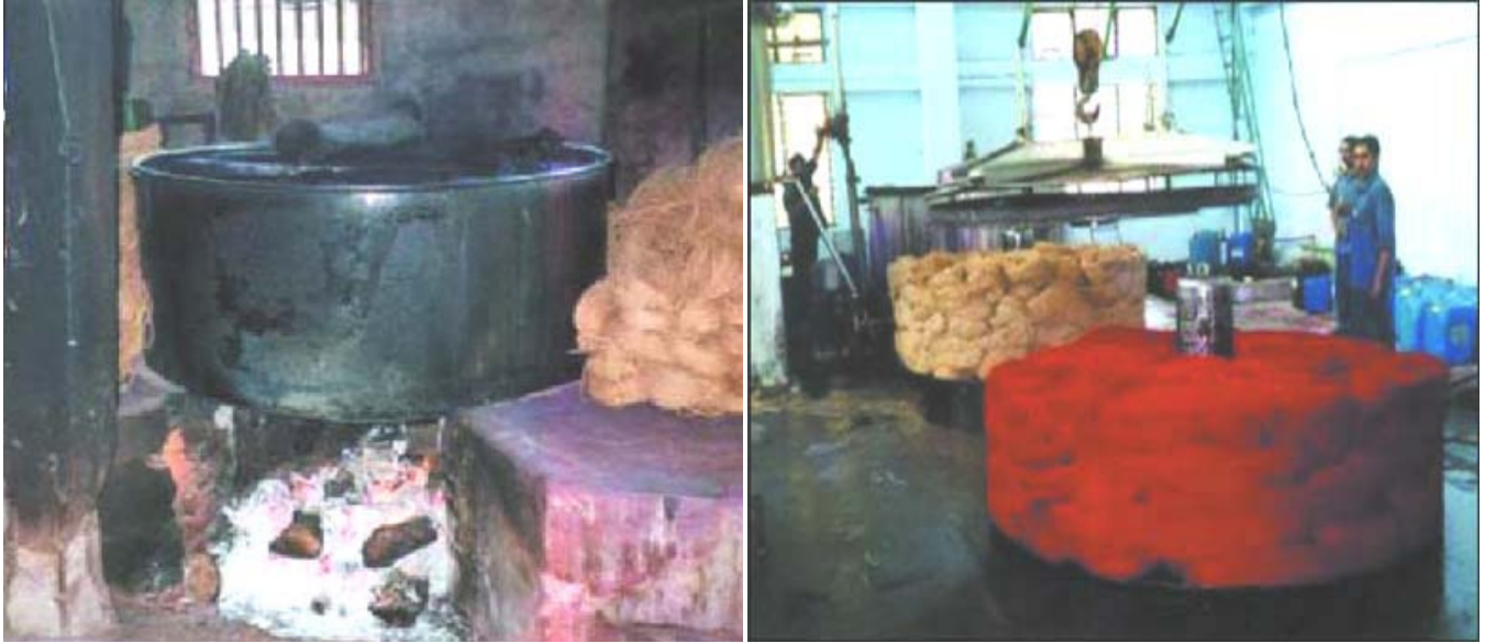
Figure-5 Traditional and Recent Dyeing Process of Coir Fiber
