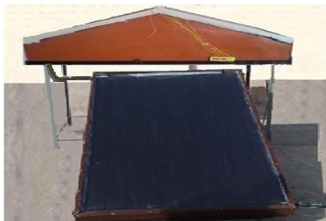
Figure-2 Double slope active solar still set up
