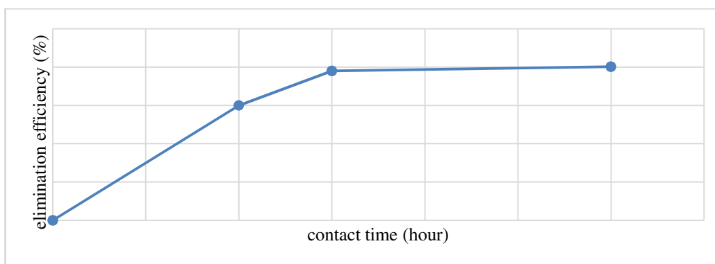
Figure-1: elimination efficiency of humic substances on raw clay as function of time.
