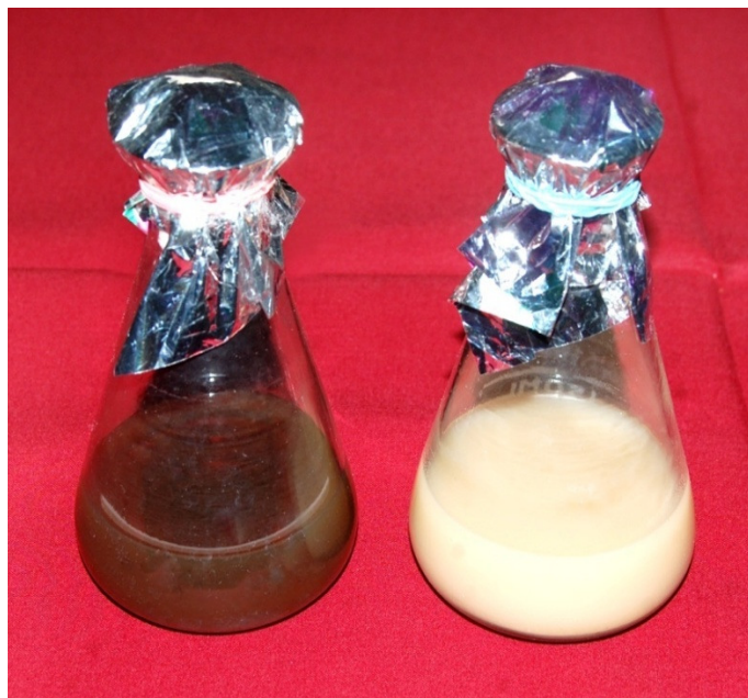
Figure-2 Oryza sativa extract before adding of AgNO 3 and The colour changes of plant extract after 6 hrs of incubation with AgNO 3
