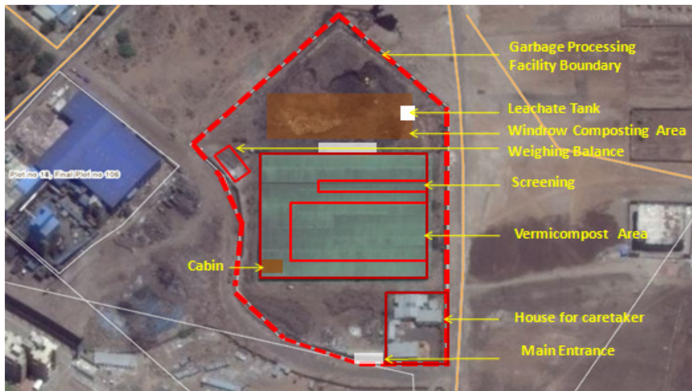
Figure-1 Layout of Garbage Processing Plant, Ramtekdi
