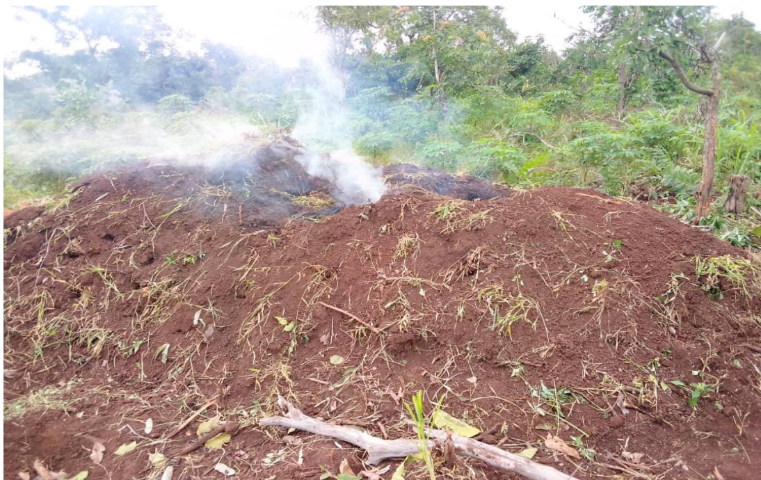
Figure-15: Earth kiln method use for charcoal production at Umogidientelkpa council.
