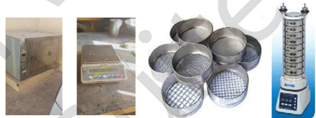
Figure-4: (a) oven, (b) scale (c) sieve.
