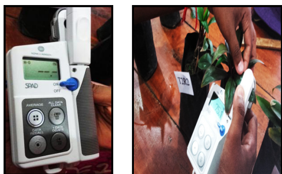
Plate-1: Measurement of SPAD value with portable SPAD502 meter.
