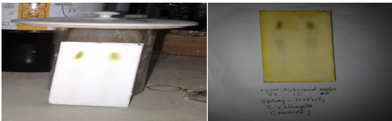
Figure-3 Thin layer chromatography observations a) Before spray of FeCl 3 and b) after spraying
